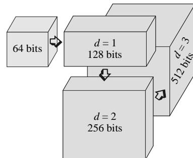
Figure 1: Construction of a three-dimensional product code with  $(8,4)$  component codes.
