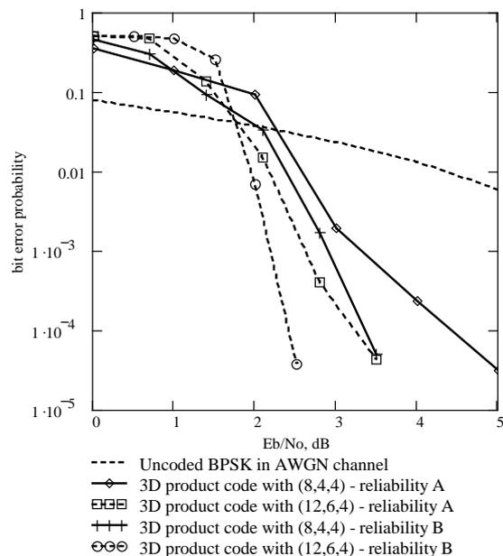
Figure 5: Performance results for the  $(8,4,4)^3$  and  $(12,6,4)^3$  product codes on AWGN channel with different reliability calculations.
