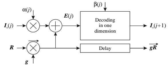
Figure 2: Decoding structure for the  $j$ -th decoding step.
