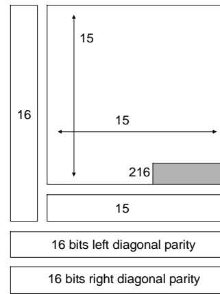
Fig. 3. Block shape matched to the specifications of DVB-RCT for QPSK ( R = \frac{3}{4} ).
