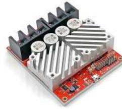
Fig. 7. Driver Roboclaw 2x60A
