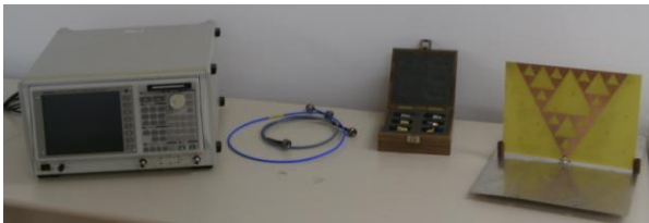
Figure 7. Antenna and equipment used to measure the return loss of the antenna in the range of 100MHz to 3.7 GHz.
