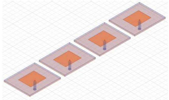
Fig. 3. HFSS model of adaptive antenna array.
