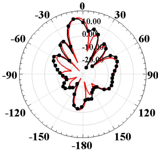
Fig. 10 Radiation pattern for  $-10^\circ$  steering angle. Continuous curve from HFSS and circle curve from optical delay line.
