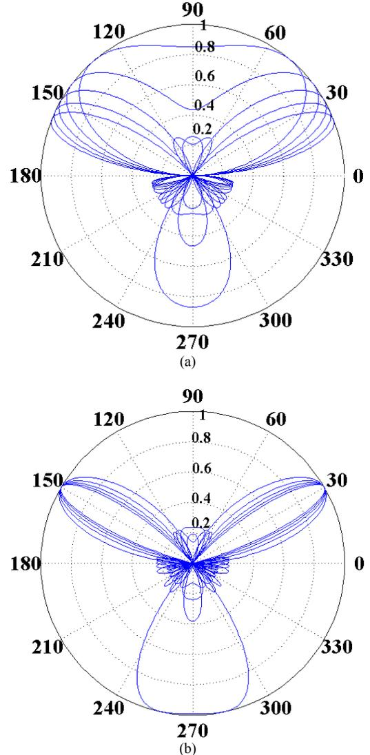
Fig. 6 Array factor of four linear and uniform array. (a) Phase shifter response. (b) Optical delay line response operating from 3.8 to 7.8 GHz.
