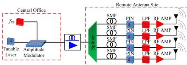
Fig. 2. Optical system diagram implemented in VPI.
