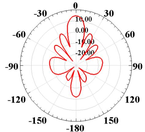
Fig. 9 Antenna array radiation pattern for x-z plan.
