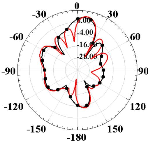
Fig. 11 Radiation pattern for  $20^\circ$  steering angle. Continuous curve from HFSS and circle curve from optical delay line
