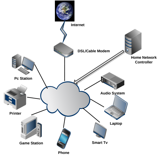
Fig. 4. Device connectivity abstraction in the SDHN.
