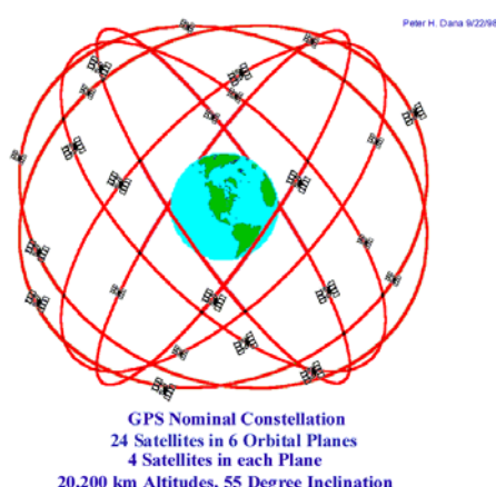
Fig.3. The GPS constellation of satellites for geopositioning.
