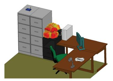
Far Field Produced by Printer Antenna 1
