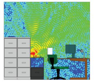
E Field Produced by Printer Antenna 1
