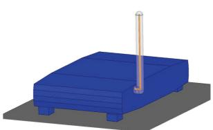
Full 3D model of Antenna Antenna Sleeve shown as transparent for clarity
