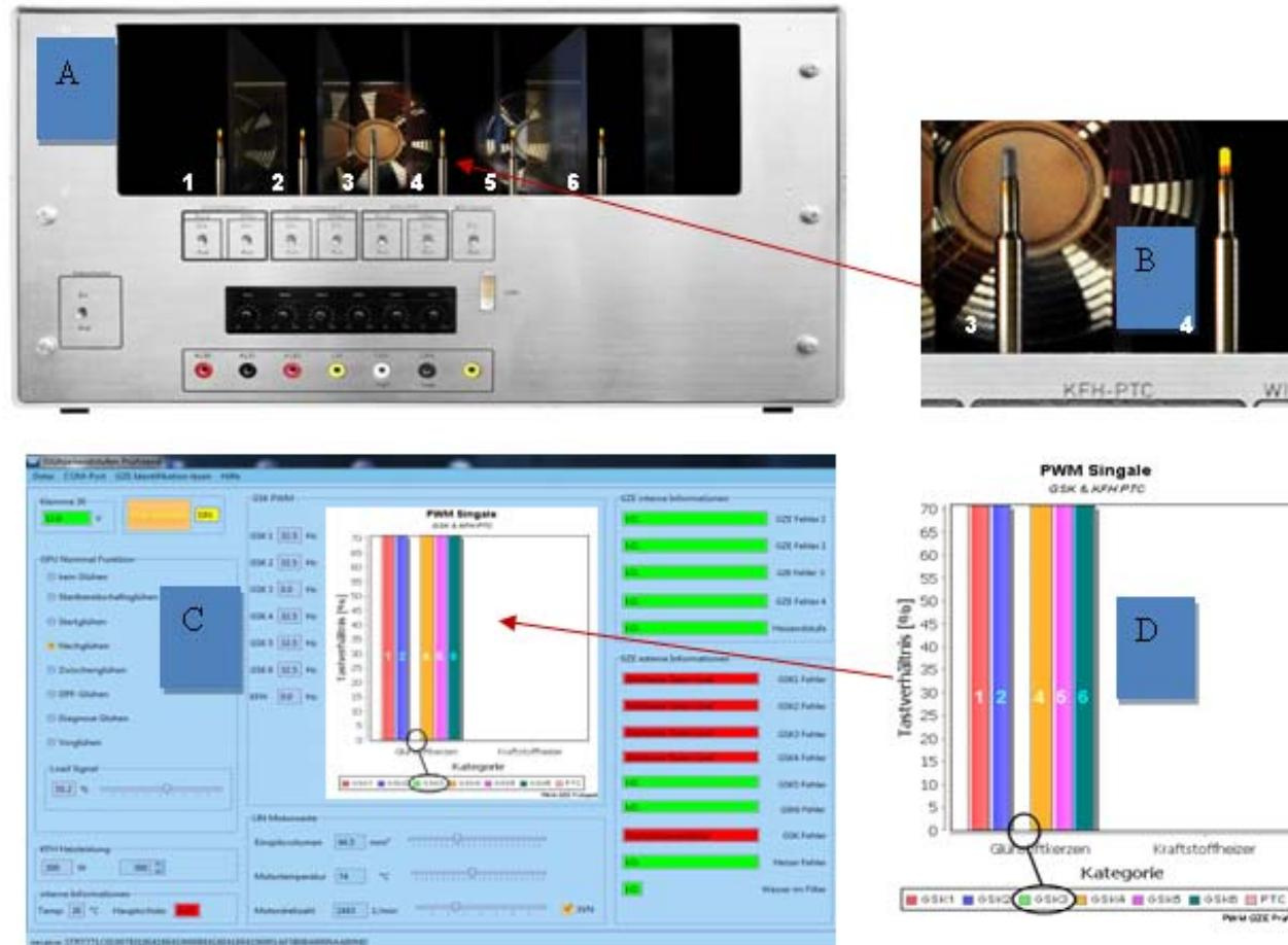
Controlled glow plugs visualized in a Graphic User Interface (GUI)
