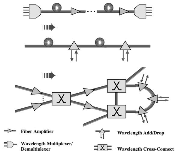
**Figure Two:** The Evolution from Photonic Transport to Photonic Networks
