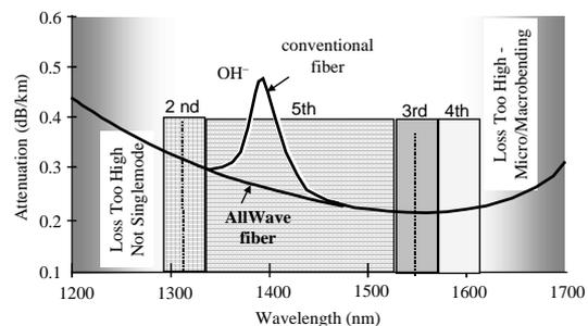
**Figure Four:** Lucent’s AllWave™ fiber eliminates the water peak, thereby increasing the number of wavelengths that can be used by more than 50%.
