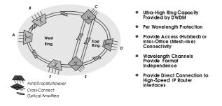
**Figure Three:** *Example of a Multi-wavelength Metropolitan Network*
