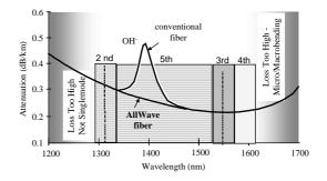
**Figure Four:** Lucent's AllWave<sup>TM</sup> fiber eliminates the water peak, thereby increasing the number of wavelengths that can be used by more than 50%.
