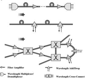
Figure Two: The Evolution from Photonic Transport to Photonic Networks
