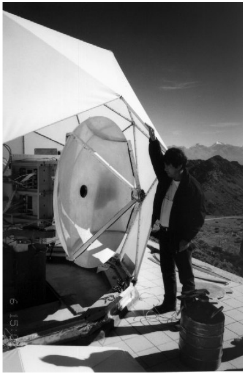
Fig. 2. The 1.5 -m submm-w cassegrain antenna seen through the radome maintenance door opening.
