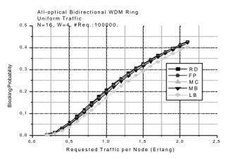
Figure 2 –Blocking probability for uniform traffic.
