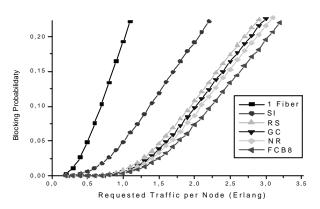
Figure 5 – Influence of upgrading the fiber plant for several levels of integration between both rings in the blocking probability on a WDM ring.
