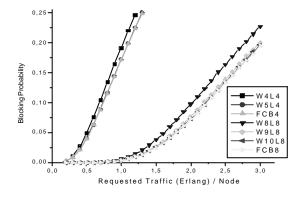
Figure 4 – Influence of upgrading the fiber load for several levels of integration between both rings in the blocking probability on a WDM ring.
