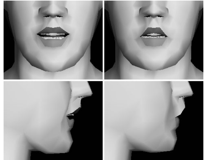
Fig. 12. The posture of the synthetic face during the production of /a/ (left side) and /u/ (right side).
