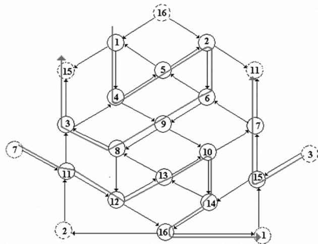
Fig. 8. OMT-16 seen as a functional ring topology.
