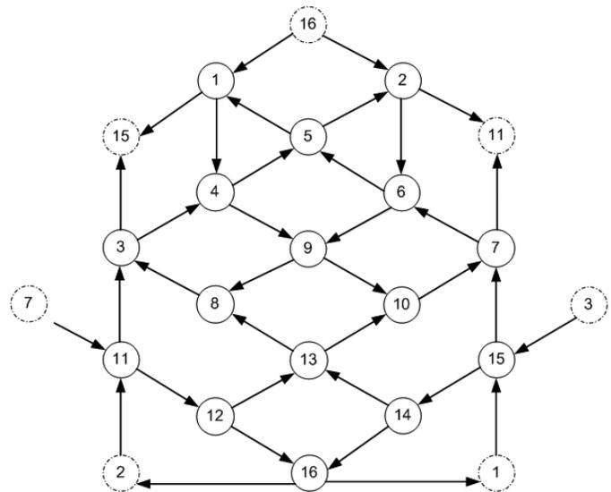
Fig. 6. An Optimized Mesh Topology for 16 nodes, OMT-16. Dashed nodes are virtual only to show connections.
