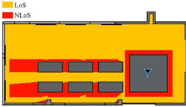
Fig. 5. Map of LoS conditions related to the AP position obtained from ray tracing simulations.
