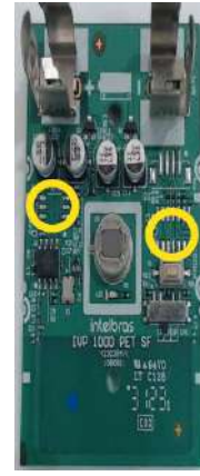
Fig. 3: Label of the CI-Missing class, highlighted by the yellow circle. This class indicates a missing IC assembly.
